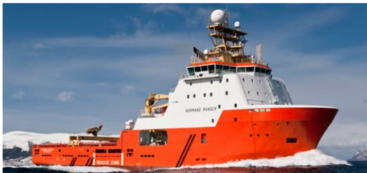
Figure 13: Normand Ranger AHTS was used to tow the assembled Hywind turbines [22]
