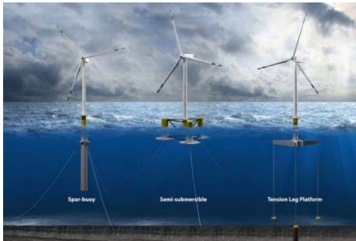
Figure 8. Floating wind concepts
